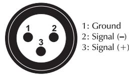
If you are using controllers with this occupation, you can connect the DMX-output of the controller directly with the DMX-input of the first fixture in the DMX-chain. If you wish to connect DMX-controllers with other XLR-outputs, you need to use adapter-cables.
