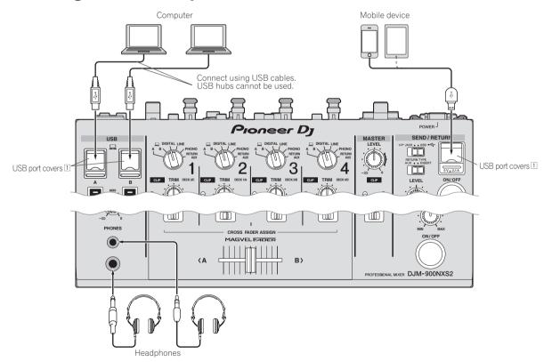
1 Do not push or pull hard on a USB port cover. It could be damaged.
